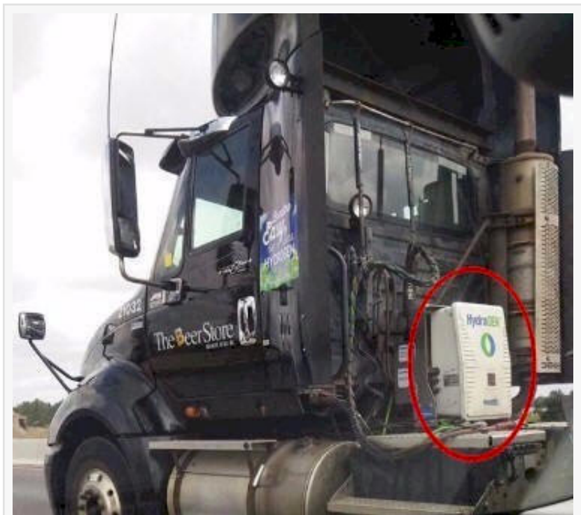
dynaCERT HG unit installed on diesel Truck
