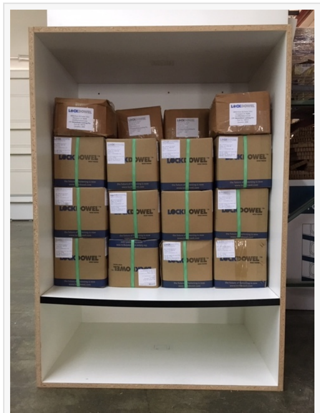
This shelf secured with Lockdowel fasteners is holding 1,164 pounds. This photo is after seven days.
