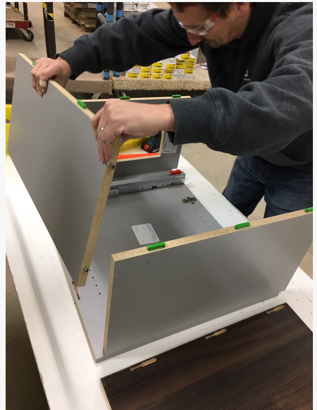
Bella IMC assembles cabinets without screws or glue using the Lockdowel system.
