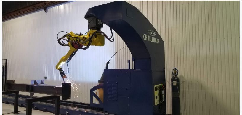
BeamMaster - Robotic Welding System Dedicated to Structural Steel Fabricators
