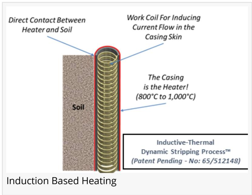
With IT-DSP™ each coil can operate at different power levels, offering unmatched regulation in vertical temperature profiles. The modular coils are engineered for sustainability and have completely reusable components. With IT-DSP™ even high boiling point compounds in challenging geology can be effectively remediated in less time, using less energy.
