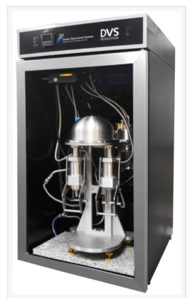
DVS Resolution by Surface Measurement Systems is a dual vapor gravimetric analyzer
