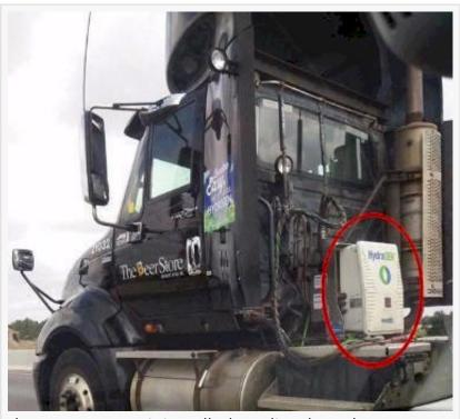
dynaCERT HG unit installed on diesel Truck
