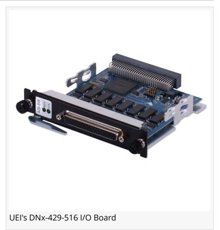
written to the ARINC 429 bus. The TX drivers on the TX/RX channels can be disabled on a channel-by-channel basis allowing TX channels to function as RX.
