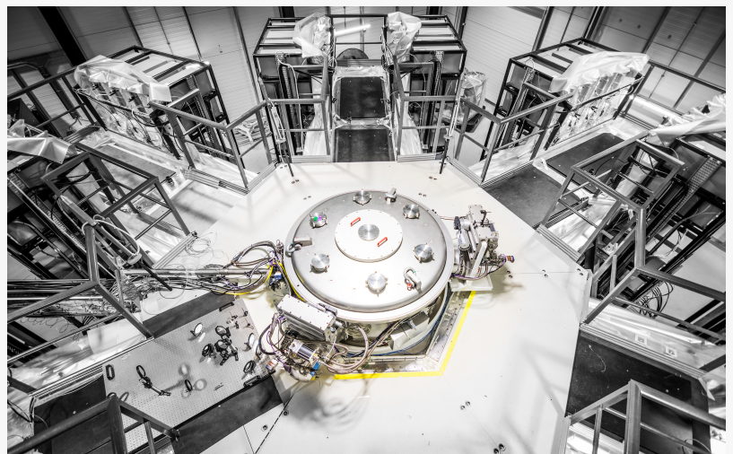
Vacuum chamber in which the firing takes place
