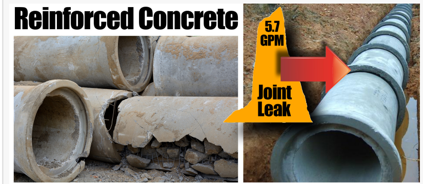
Reinforced Concrete Pipe testing using FELL technology.
