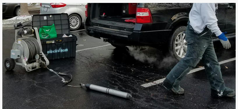
Electro Scan's ES-620 Portable configuration designed for difficult access and remote pipeline assessment.
