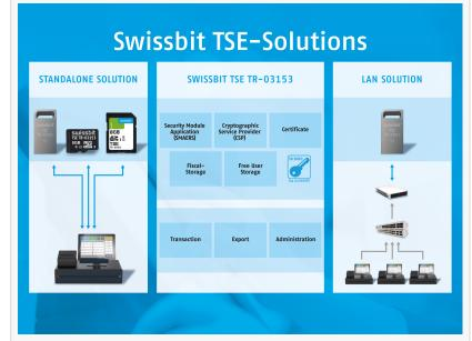
The TSE from Swissbit is available as a standalonedevice solution as well as a LAN solution with multiple parallel TSEs that connect different devices.
