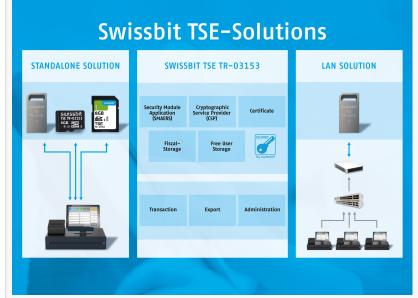
The TSE from Swissbit is available as a standalonedevice solution as well as a LAN solution with multiple parallel TSEs that connect different devices. system without the need for hardware upgrades of each individual cash register.
