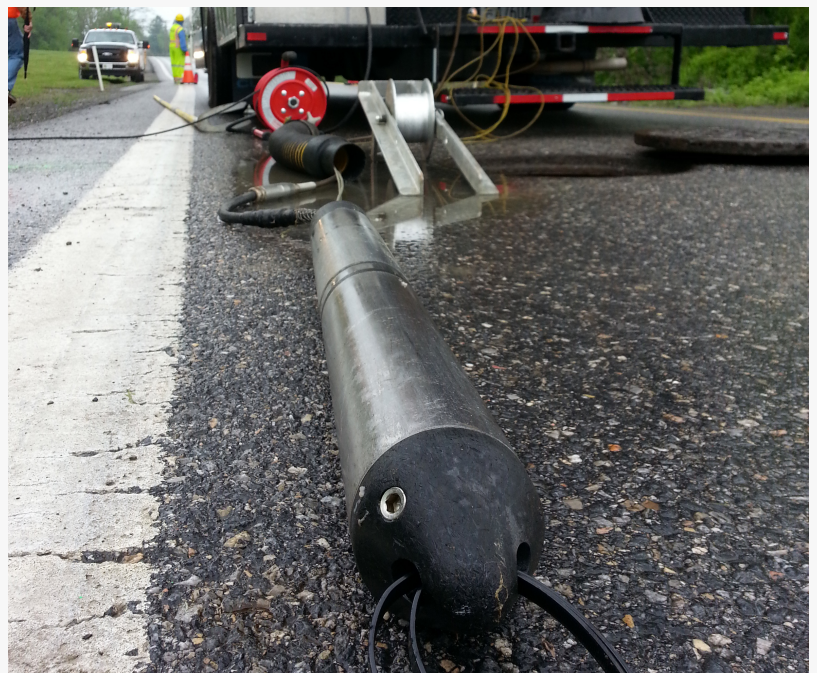
Electro Scan Ruggedized Machine-Intelligent Pipeline Assessment Probe.
