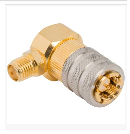
style of coupling used by this SMA adapter does not require any tooling for mating or unmating. This right angle adapter offers excellent electrical performance through 20 GHz and is constructed with a gold plated, brass body.
