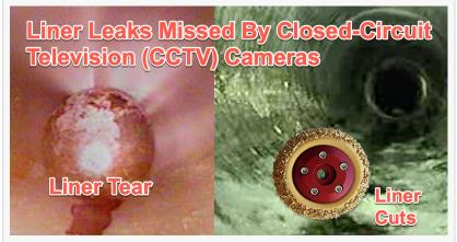
Leaks in CIPP liners missed by Closed-Circuit Television cameras which cannot determine watertightness.
