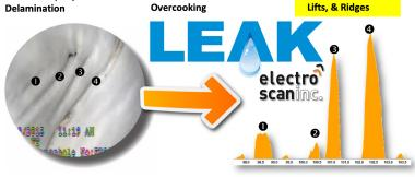
CIPP leaks not seen by visual inspection or CCTV cameras.
