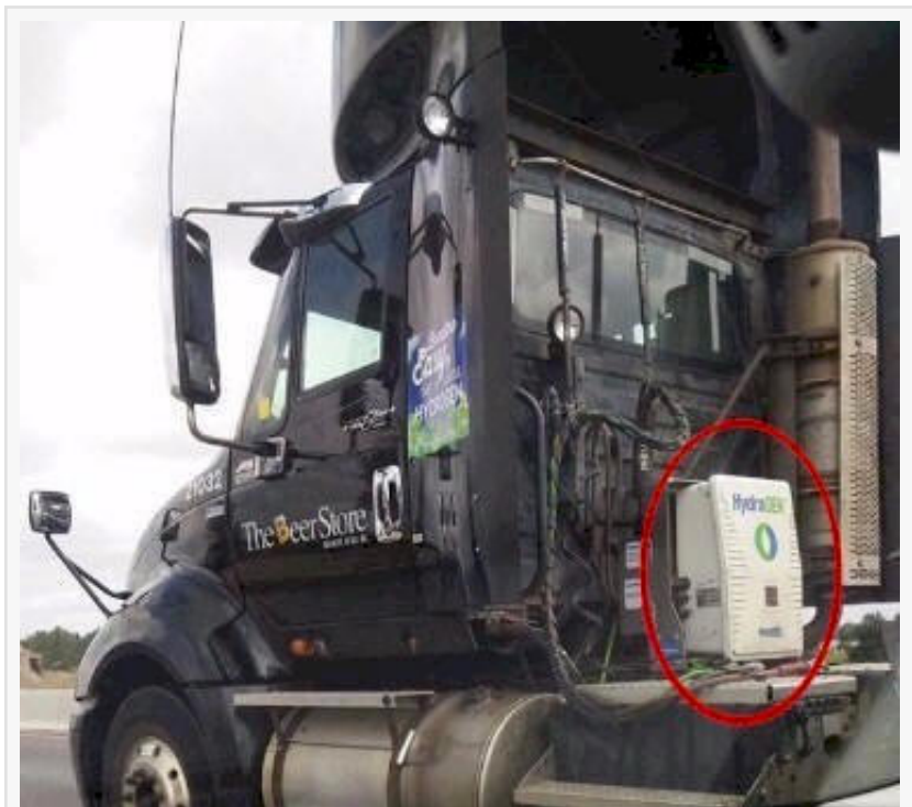
dynaCERT HG unit installed on diesel Truck
