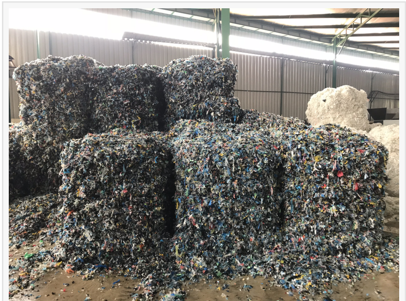
Shredded and sorted thin film plastic - prepared for recycling
