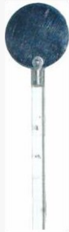
Circular Disk in Plastic Handle, Proof Plane, for Removing Static Electricity
