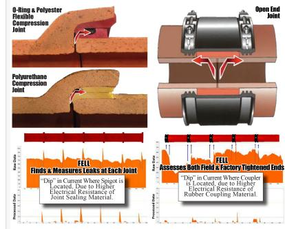
Electro Scan's patented technology can locate leaks in new & existing Vitrified Clay Pipes, including compression joints and open ended joints.
