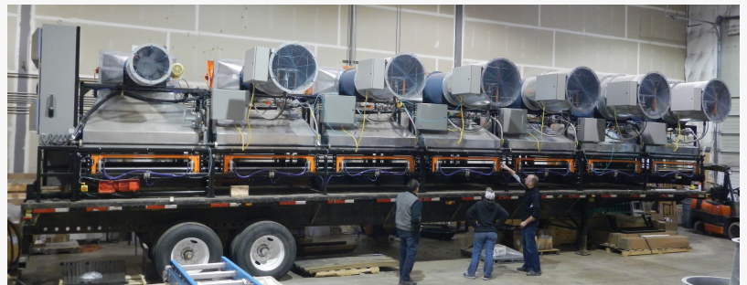
Mobile Hemp Dryer
