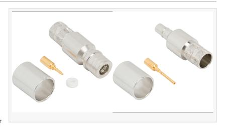
The new connectors are available in both straight plug and jack configurations and operate at 50 ohms with a frequency range of DC to 12.4 GHz, which exceeds the maximum frequency supported by the cable of 8 GHz. These connectors feature a traditional snap-on interface for quick and easy installation and low RF leakage. QMA connectors are ideal for applications such as 5G wireless, medical and test and measurement.
