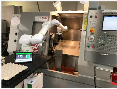
Productive Robotics' OB7 CNC Package comes fully equipped with all the accessories needed to connect to any type of CNC Mill, Lathe, or other machine.
