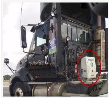
dynaCERT HG unit installed on diesel Truck
