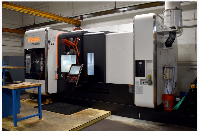
New Mazak Integrex i-400 5-Axis Machining Center Installation at Trace-A-Matic North
