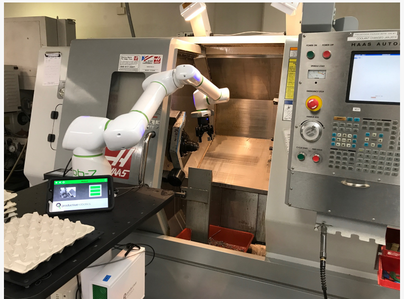
With 7 axes or degrees of freedom, OB7 is ideal for automating CNC machine tending, packaging, palletizing, plastics injection molding, and many and other manufacturing applications..
