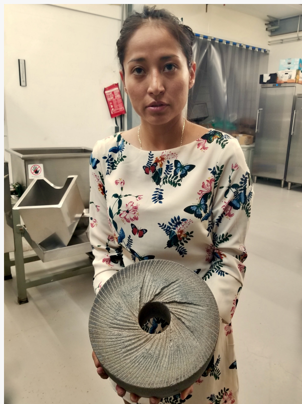
Karla Plancarte, owner of "Tortillería Taiyari," shows the volcanic stone she uses to grind the corn into flour.
