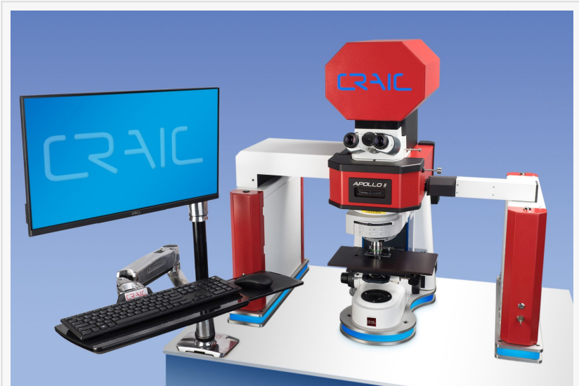
CRAIC UV-Vis-NIR and Raman Microspectrometer
