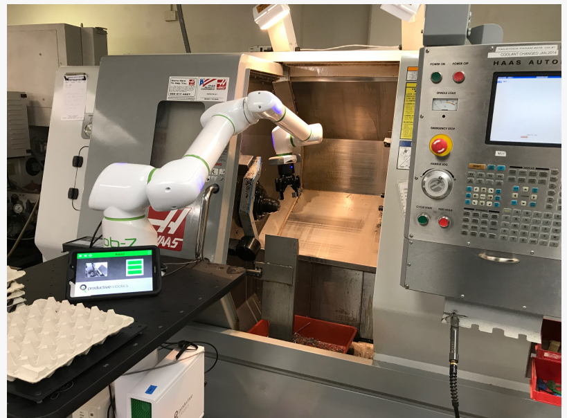
OB7 can be used for all sorts of manufacturing tasks, including CNC machine tending.
