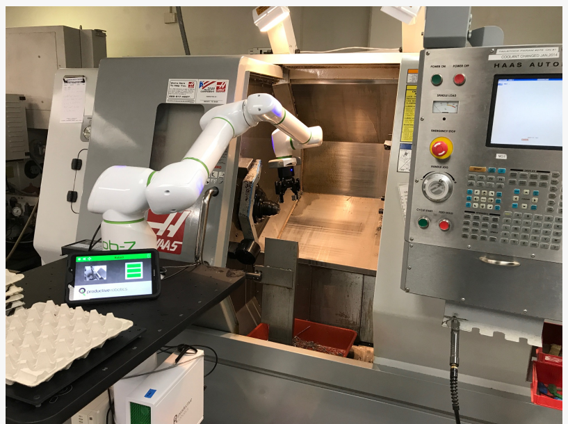
OB7 Cobot Machine Tending Package comes included with all the necessary equipment to get started automating CNCs.
