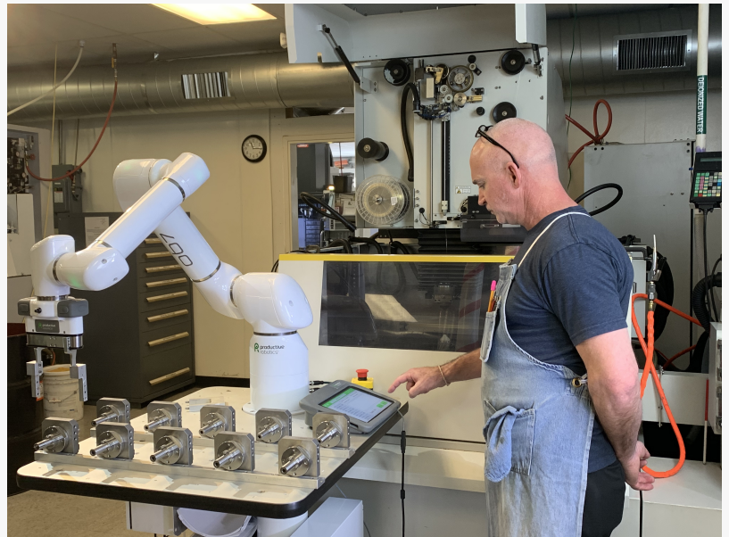
OB7 Machine Tending Cobot loads and unloads parts on a Wire EDM Machine.
