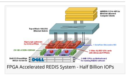
Field Programmable Gate Arrays (FPGAs) are drastically increasing the speed of database servers. By implementing a Key-Value Store (KVS) entirely in FPGA logic, servers can offload time-critical queries from the CPU. In this work, we describe the architecture of a 1U server that uses an AMD CPU to implement a full REDIS database coupled with three Xilinx® FPGA-based Alveo™ U50 accelerator cards that offload 450M GET or SET Input/Output operations per second (IOPs).
