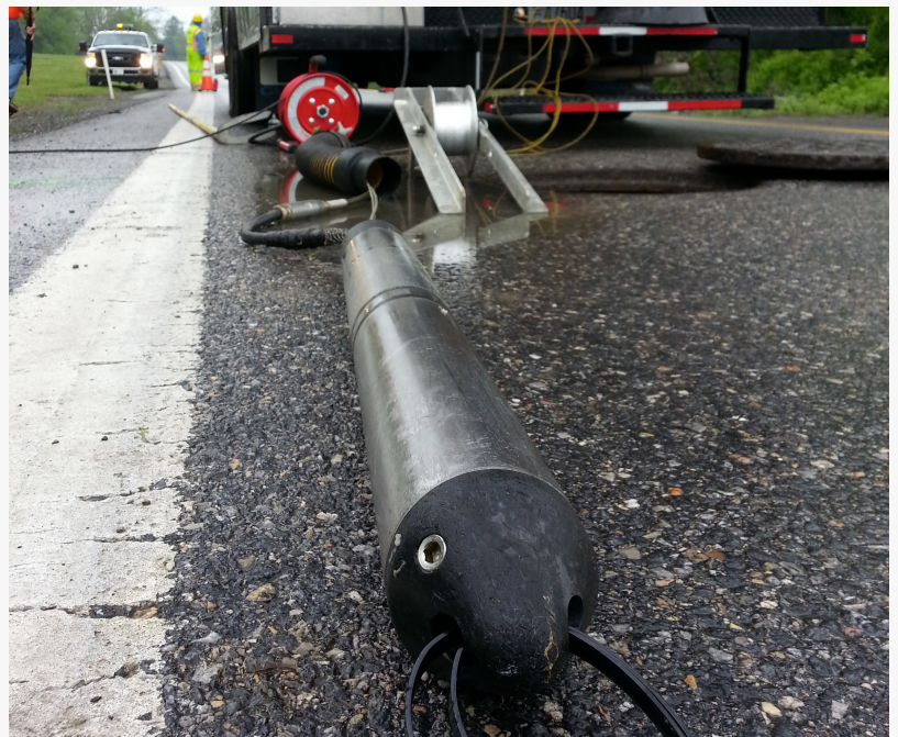
Electro Scan ruggedized machine-intelligent pipeline assessment probe.
