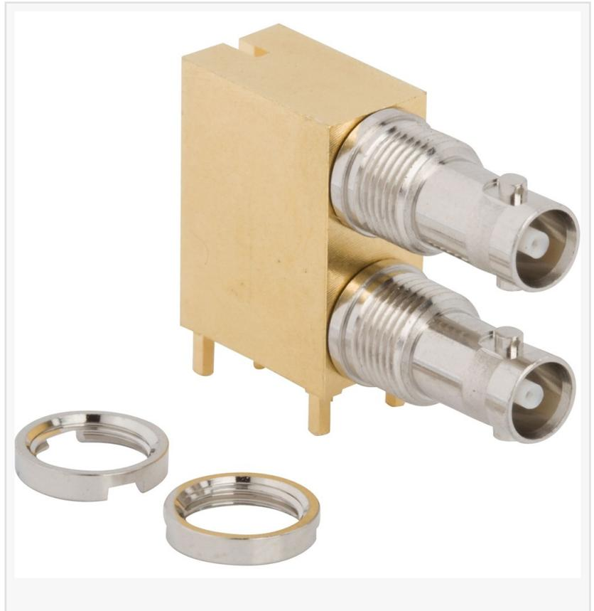
The HD-BNC dual port PCB jacks feature the popular bayonet style coupling mechanism and offer stable electrical performance through 18 GHz. The connector contacts are gold plated beryllium copper, and bodies are matte tin plated zinc die-cast, or gold plated machined brass. Both designs have a secure bulkhead mounting feature. These jacks are available as both stacked and staggered mount configurations for additional versatility.
