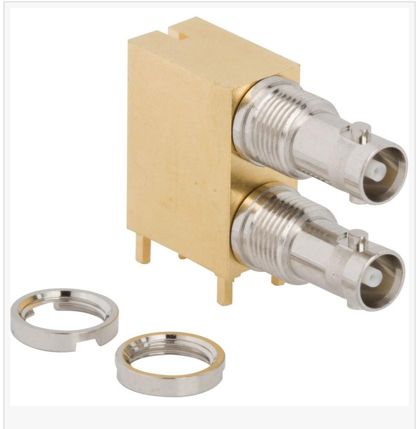
The HD-BNC dual port PCB jacks feature the popular bayonet style coupling mechanism and offer stable electrical performance through 18 GHz. The connector contacts are gold plated beryllium copper, and bodies are matte tin plated zinc die-cast, or gold plated machined brass. Both designs have a secure bulkhead mounting feature. These jacks are available as both stacked and staggered mount configurations for additional versatility.
