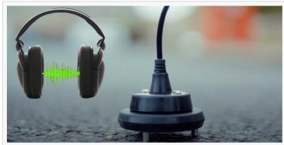
Acoustic listening devices attempt to triangulate leak locations on metallic pipes, but problematic in testing for leaks in plastic pipes that have become more common.
