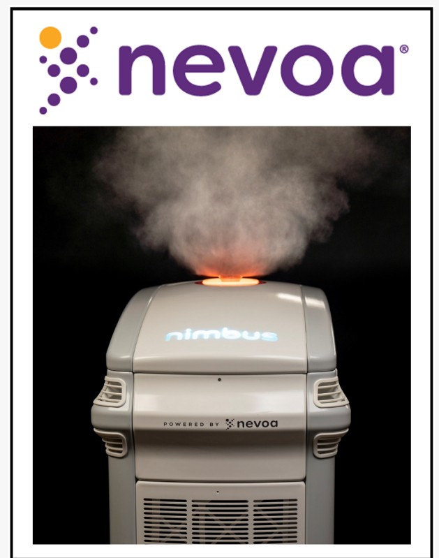
Nimbus, a disinfecting robot by Nevoa Inc., fogs Nevoa Microburst Solution to disinfect patient rooms, killing 99.8% of pathogens such as coronavirus.
