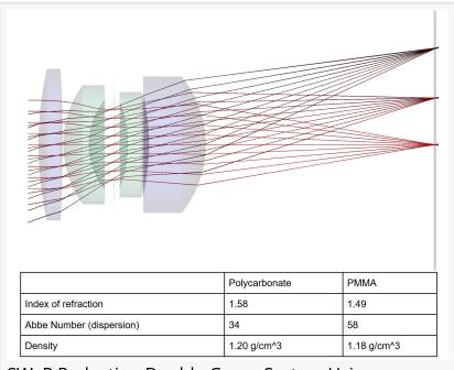
SWaP Reduction Double Gauss System Using Gradient Index
