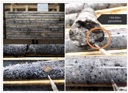
Drill core from NioBay's Winter-2020 drill program at the James Bay Niobium Project. Note the size of the pyrochlore, which is the mineral that contains the Niobium
