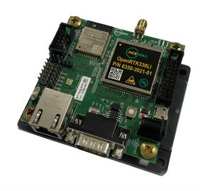
The OpenRTK330L utilizes a very precise 2 Degree/Hour IMU to offer ten to thirty seconds of high accuracy localization during full GNSS denial. This enables autonomous system developers to safely deliver highly accurate localization and position capabili
