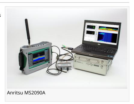
Anritsu Company and COMINT Consulting announce the compatibility of the COMINT <a href="Krypto1000">Krypto1000</a> Wideband Signal Analysis and Decoding Suite with IQ data captured with the Anritsu Field Master Pro™ MS2090A handheld real time spectrum analyzer (RTSA). The MS2090A performs capture and streaming of up to 110 MHz of IQ bandwidth across full 54 GHz, providing a broader range of RF IQ data for post processing to deliver a deeper view of SIGINT and/or COMINT activity.
