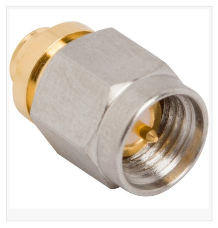
various conformable and semi-rigid cables. A threaded coupling mechanism ensures uniform contact of the outer conductors which enables the SMA connector to minimize reflections and attenuation at higher frequencies. This allows for a high degree of mechanical strength and durability.
