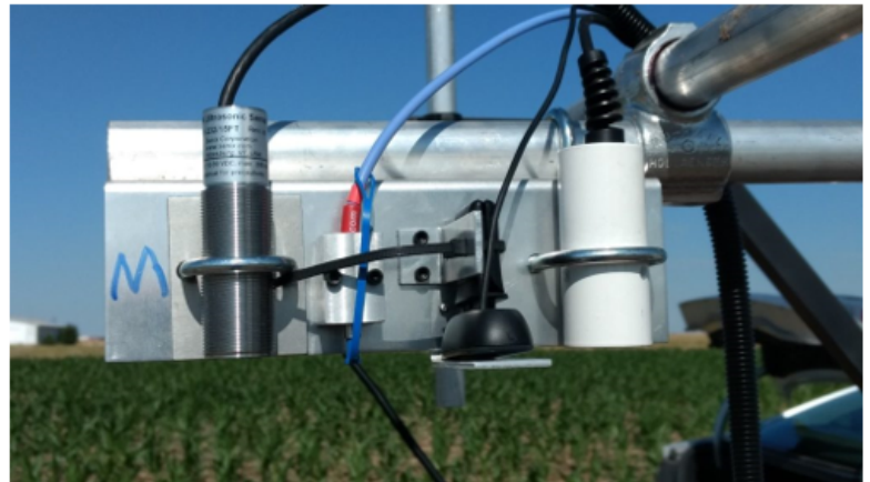
The Senix ToughSonic 14 on the left, pointed down at the crop canopy along with other sensors
