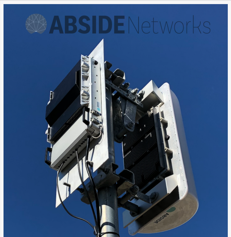
Abside Networks Gen3 LTE eNB powered by Amarisoft's software technology and serving non-3GPP frequencies
