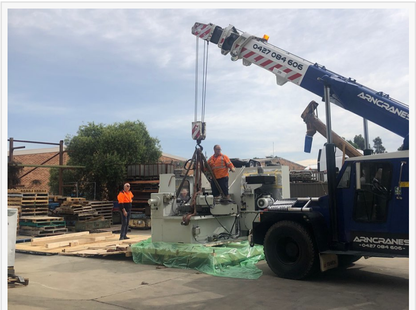
New Leifeld CNC Spinning Machine Being Unpacked
