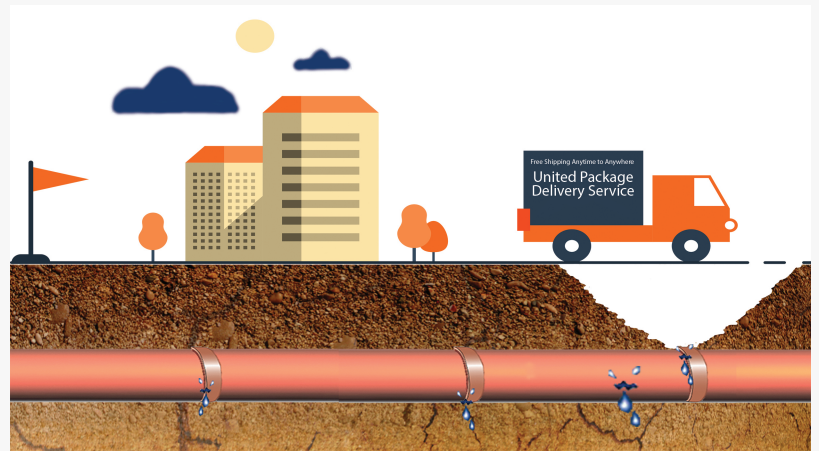
Surcharged pipes often seep effluent through defective joints outside of the pipe. Liquified soil then re-enters the pipe through joints causing silt to accumulate at the bottom of the pipe and a creating a void above the pipe's crown.
