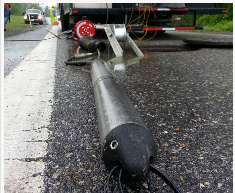
Electro Scan ruggedized machine-intelligent pipeline assessment probe.
