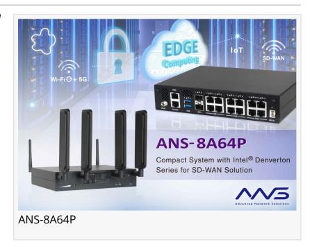
ANS-8A62P C3558 (4C) or high performance ANS-8A64P C3758 (8C) appliance. Both appliances are designed and built with <u>SD-WAN (SDN)</u> applications in mind for deployment in 5G and IoT devices.
