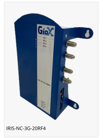
fiber network, the solution is also used for mobile backhaul. The company's IRIS<sup>™</sup> product line consists of network controllers and CPE and offers a means to re-use the in-building coax networks to offer symmetrical broadband services well beyond the 1Gbps.
