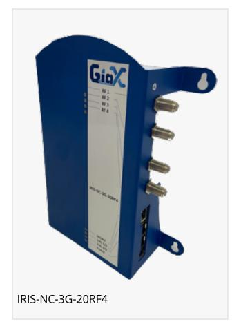
backhaul. The company's IRIS<sup>™</sup> product line consists of network controllers and CPE and offers a means to re-use the in-building coax networks to offer symmetrical broadband services well beyond the 1Gbps.
