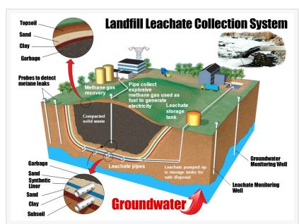
Landfills must contain all potential runoff or leachate using undergound piping, storage ponds, and tanks.
