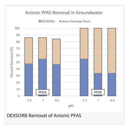
hydrophobic and electrostatic adsorption to  $\beta$ -cyclodextrin cups and cationic quaternary ammonium sites. Dual binding allows DEXSORB+ to uniquely address the structural variances of chain length, functional groups, and isomer structures among PFAS.
