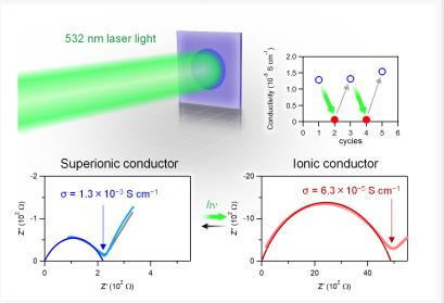
lonic conductivity (σ) switches by irradiating 532 nm laser light, and returns to the original value with time. This photoswitching effect is repeatedly observed.
