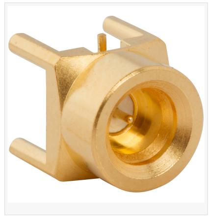
Higher frequency performance can be reached through PCB optimization analysis using readily available HFSS 3D models. They are constructed using machine brass bodies and contacts on all receptacle interfaces, and available in both smooth bore and limited detent mating configurations.
